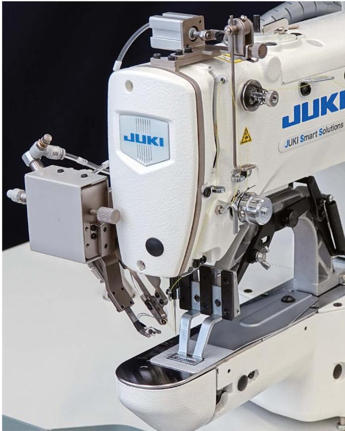
Needle thread clamping mechanism
