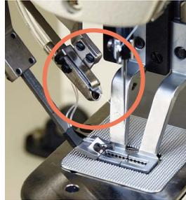
It holds the needle thread after thread trimming and prevents the needle thread from getting caught on the back side of the fabric.
