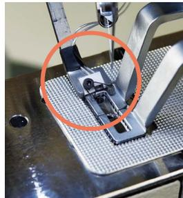
Newly adopted heat cutter can cut from thin thread to thick thread.
