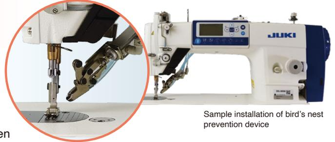
Sample installation of bird's nest prevention device
