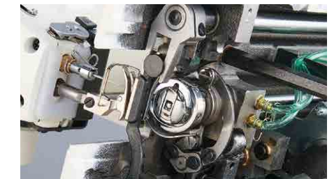
Lower side of the thread-trimming knife
