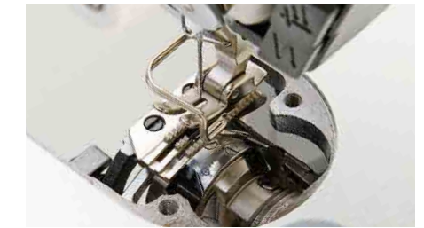
Upper side of the thread-trimming knife
