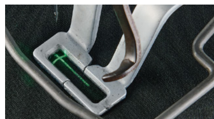
Example of The H type thread guide installed.
