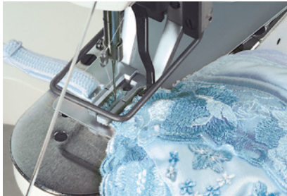
F type (Attaching the shoulder straps to brassier)
