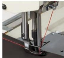
The lineup includes a CS-specification model for sewing car seats. Changes have been made to the thread take-up lever stroke and feed motion to further improve sewing quality in seat sewing.
