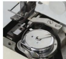
The meshing of the fixed knife and the moving knife linearly moving in parallel with the feed dog enables excellent cutting of thread from thin to thick threads (#8).
