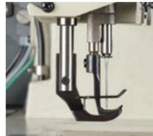
For easier insertion and removal of thicker materials, a reverse needle raising function is available. This function reverses the needle back after thread trimming to ensure a lifting height of 16 mm for the presser.
