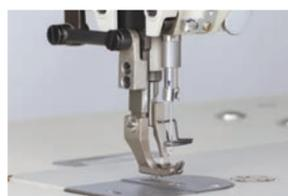
**Top and bottom feed mechanism for reliable feeding**
