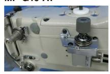
Upper thread break detection equipment MP-G10-TS
