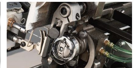
Lower side of the thread-trimming knife
