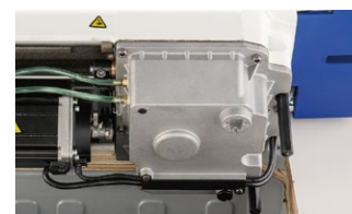
Oil-shielded made of aluminum die cast
