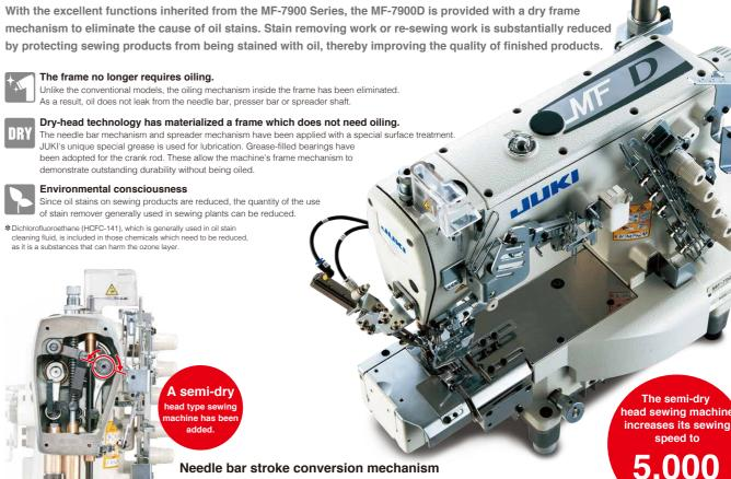
By changing over the needle bar stroke, penetrating force of the needle as well as thread tension to fit heavy-weight materials (fleece, blankets) can be obtained. The needle bar stroke can be changed by adjusting the eccentric pin. (Changing of parts is not required. Factory-set at the time of delivery: 31mm; for sewing heavy-weight materials: 33mm)
