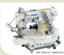
The machine can be used for the hemming process of the sleeves and bottoms of T-shirts and for the covering process for sportswear and knitwear.
