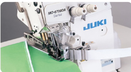
● Rolling in tape MO-6745DA-FF4-360/N077 (N077: Clean finish top and bottom)
