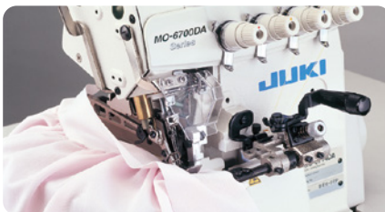
● Gathering MO-6714DA-BE6-327/S162 (S162: Swing-type gathering device, manual-lever operated)
