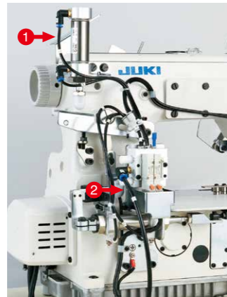
1 Presser lifter drive mechanism air cylinder 2 Thread trimmer drive mechanism air cylinder
