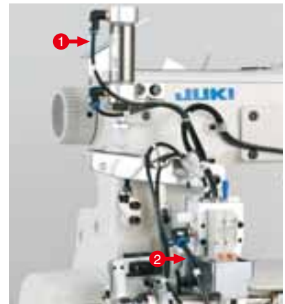
① Presser lifter drive mechanism ② Thread trimmer drive mechanism
