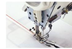
The sewing machine provided with an anti-material-slip function, which promises more beautifully finished seams, is included in three different model lineups.
