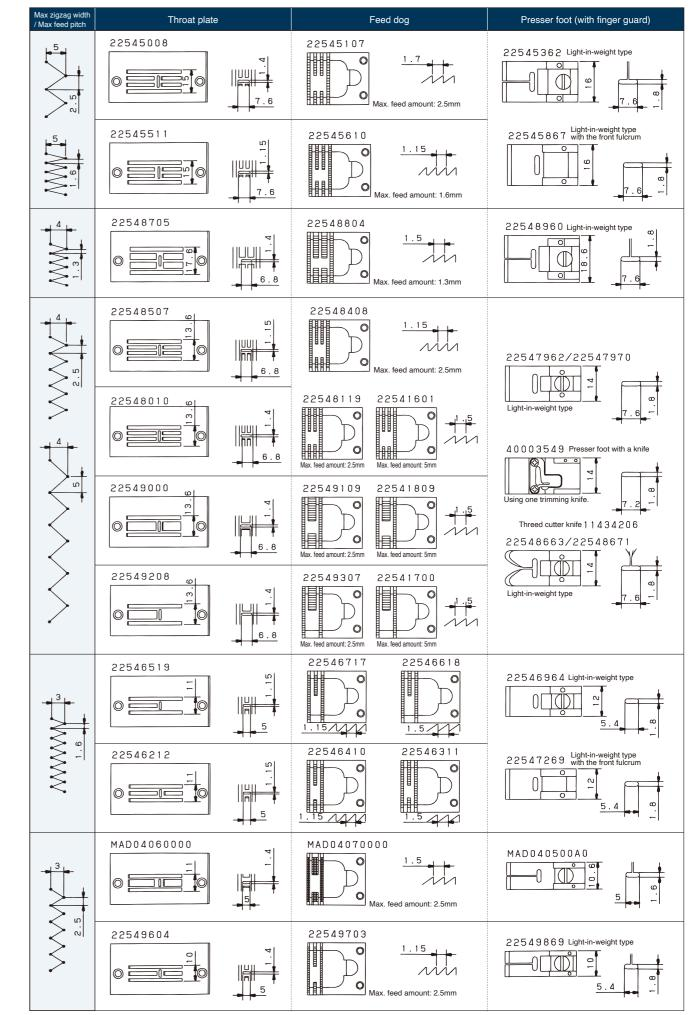
Two different part numbers are assigned to one presser foot (ex. 22547962 and 22547970), if you place a order for 22547962 (left number), factory supplies you presser foot installed with a big figure guide, 22547970 (right number) with small finger guide respectively.
