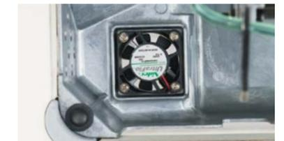
The cooling fan is laid out at the position that is best to reduce the heat generated by the hook unit.
