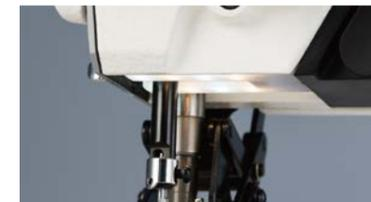
The LED light is provided as standard on the undersurface of arm jaw. In addition to the conventional function of the LED light, the color shade can be changed over as "white ⇄ neutral color (initial value) ⇄ incandescent" so as to help reduce the operator's eye fatigue.
