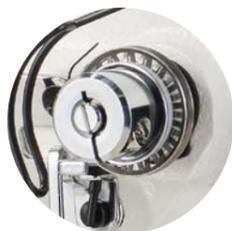
The LZ-2290C is the world's first sewing machine that comes with the rotary-type active tension. Conventionally, it has been difficult to adjust the thread tension when the remaining amount of bobbin thread has reduced. This sewing machine, however, is able to correct and stabilize the thread tension by means of the active tension. In addition, the thread tension can be corrected according to the sewing speed, thereby contributing to improved seam quality.
