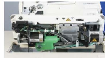
The semi-dry machine head that is supplied with grease has been developed. With this machine head, oil stains on sewn products are reduced.
