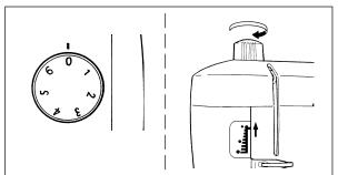
Rotate presser foot pressure regulator until blue bar in pressure indication window is at top.
