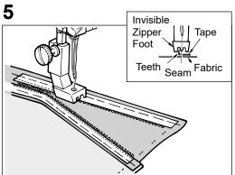
Sew the remaining zipper tape on the other side of seam allowance in the same procedure. (The lower portion of zipper tape located below the bottom of the opening will remain loose without sewn on the seam allowance.)
