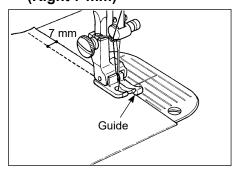
Sew the material while aligning its edge with the guide.
