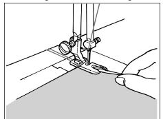
Fit the material into the vortex groove in the hemming foot until the descended needle reaches the material, and lower the hemming holder.
