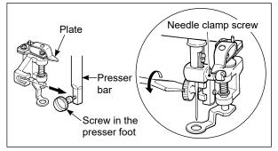
Put the plate on the needle clamp screw, insert the installing portion into the presser bar, and securely tighten the screw in the presser foot.
