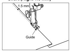
By guiding the fabric along the guide, stitching can be sewn 1.5 mm from the guide.
