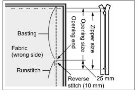
Place two pieces of fabric face to face. Baste the fabric from the edge of fabric to the opening end. At the opening end, change the stitch length to [2.0] and sew reverse stitches by 10 mm and sew until the predetermined position is reached. Neatly open the seam allowance.
