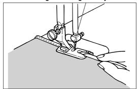
Draw the needle and bobbin thread ends with your left hand, turn the handwheel by 3 or 4 rotations until you are sure that the material edge is rolled into the groove.
