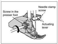
Fit forked portion of the actuating lever to the needle clamp, insert the installing portion into the presser bar, and securely tighten the screw in the presser foot.
