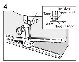
Aligning the teeth of either zipper tape with the groove on the zipper foot, sew the zipper at the very edge of the teeth from the end of opening while raising the teeth with fingers.
