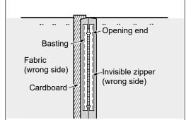
Put the invisible zipper on the fabric so that its center meets the seam line. Place a cardboard between the seam allowance and front fabric. Manually baste both sides of seam allowances and zipper tapes. Upon completion of basting, remove the cardboard.
