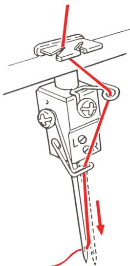
**6 mm wide 3-thread Overlocking** (Left-hand needle) (Blue, red and yellow)
