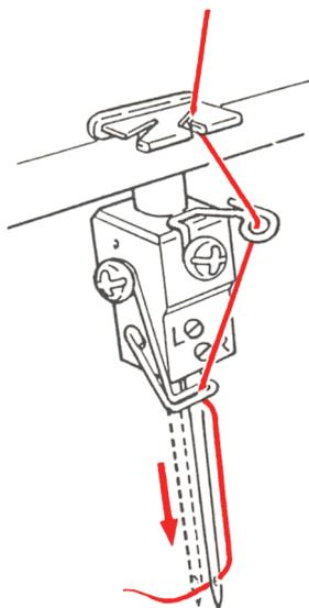
**4 mm wide 3-thread Overlocking** (Right-hand needle) (Blue, red and green)
