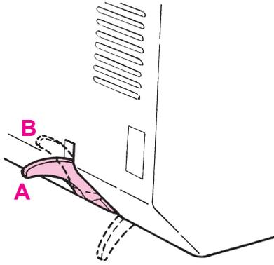
**Presser foot lifter** (To raise the presser foot by the presser foot lifter)
