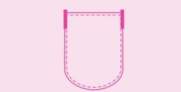
Slightly hold the end of the upper thread and start sewing. Bar tack stitches are sewn.
