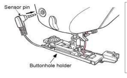
If you start the machine without inserting the sensor pin of the "buttonhole holder" into the hole completely, you will see the following message appear on the display for an instant.
