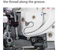
Slit-Type Molded Looper Threading Paths
