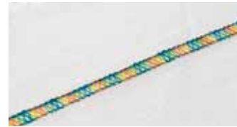
3-Thread Flatlock Use this stitch as an accent on clothes, interior items and accessories.
