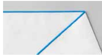
3-Thread Rolled Hem The fabric edge is rolled, then covered with thread.
