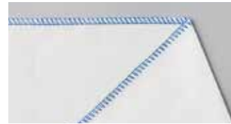
2-Thread Overcast Simply sew fabric edges with 2 threads to prevent fraying.
