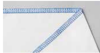
3-Thread Overlock This basic stitch of sergers prevents fabric from fraying.
