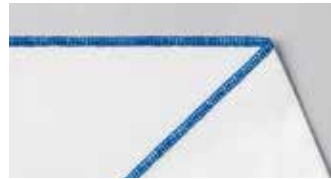
3-Thread Narrow Overlock The fabric edge is rolled, then sewn with very narrow overlocking.
