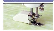
With its reliable feed, the even feed foot ensures the machine's ability to produce beautiful seams when sewing difficult-to-feed fabrics such as georgette and velvet, as well as heavy weight materials such as leather. The even feed foot is ideal for sewing multiple layers of fabric evenly.
