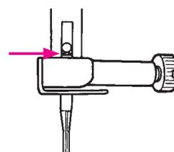
It is impossible to perform stitching if the needle is not correctly installed or a bent needle is used. Pay close attention as this will cause machine malfunction.
