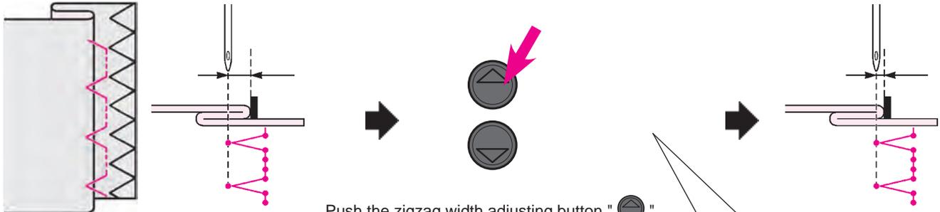
Push the zigzag width adjusting button "▲".
