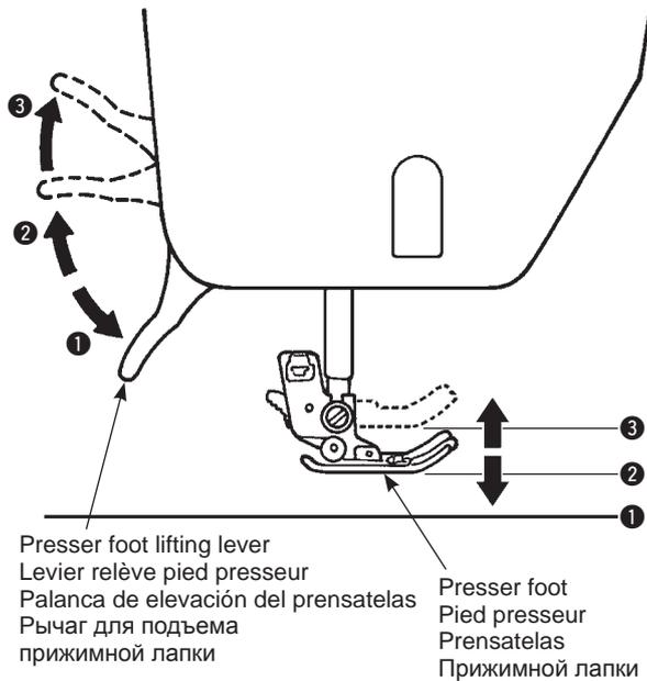
The presser foot can be up or down position by using the presser foot lifting lever.
