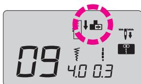
\* The icon on the screen will disappear when the lever is correctly set.
