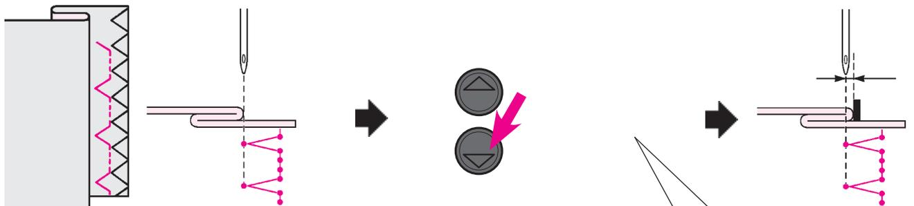
Push the zigzag width adjusting button "▼".
