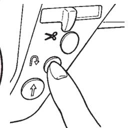
● **When the machine comes to the sewing end point, push the reverse stitch button.**
