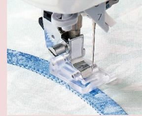
Since the front and back of this presser foot are short and transparent, appliqués and designs are easy to see, and you can easily sew sharp curves.
