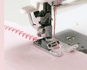
The groove along the bottom of this presser foot ensures that the presser foot does not catch on the stitching, so the fabric will be smoothly fed.
