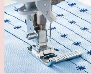
On the right side of the presser foot, there are guidelines at a 2 mm spacing from 0 to 2 cm from the center of the needle entry opening (center needle position).
