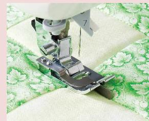
The long guide at the center of the presser foot fits perfectly in the seam line to stabilize stitching.
