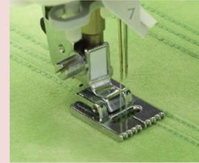
When sewing pintucks in parallel, the 9 slits on the bottom of the presser foot can be used as a guide.
