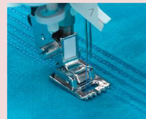
When sewing pintucks in parallel, the 7 slits on the bottom of the presser foot can be used as a guide.
