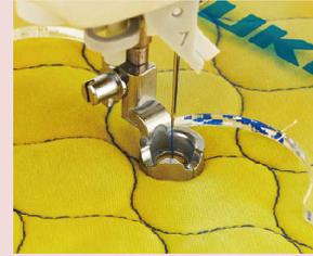
With a distance of 1/4" (6.5 mm) from the needle entry point to the outer edge of the presser foot, sew using a ruler as a guide. The front of the presser foot is lowered, making it easier to see the needle area. Adjust the height of the presser foot according to the thickness of the fabric.
