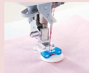
Be sure to first lower the feed dog so the fabric is not fed and adjust the zigzag width so the needle enters the holes in the button.
