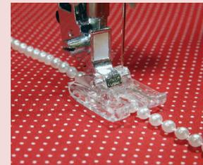
Pass the strand of pearls or beads up to a diameter of 4 mm through the dome-shaped groove in the center of the presser foot, and then sew with a zigzag stitch.
