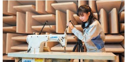
Noise rating in a semi-anechoic chamber
