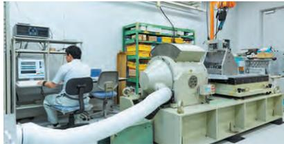
Vibration test using a vibration exciter
