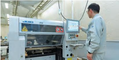
Durability test for a chip mounter
