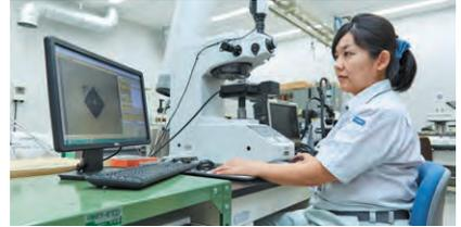
Hardness test using a Vickers hardness tester
