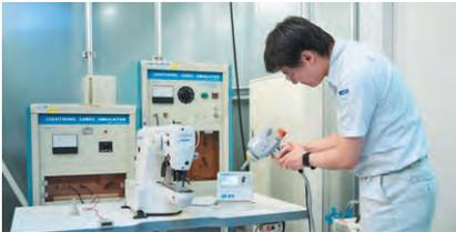
Test using an electrostatics tester
