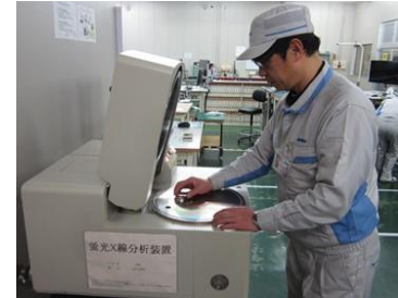
Provide testing for harmful substances using X-ray fluorescent (XRF) analyzers
