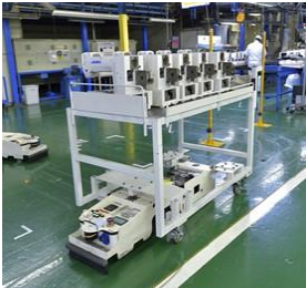
Achieve more efficient production using automated guided vehicle systems in between production procedures
