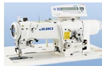
High-speed, 1-needle, Lockstitch, Zigzag Stitching Machine LZ-2280A Series (Authorized in July 2013) Click here for product details
