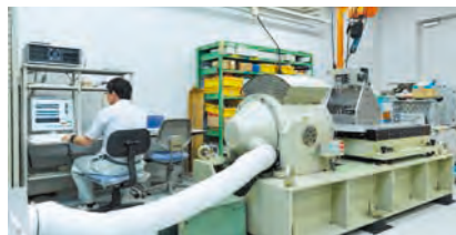
Vibration test using a vibration exciter
