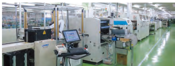
Model line automating the manual mounting work in the post-process
