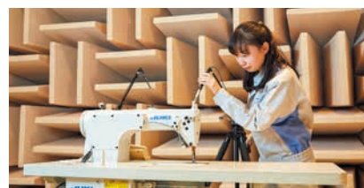
Noise rating in a semi-anechoic chamber
