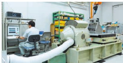
Vibration test using a vibration exciter
