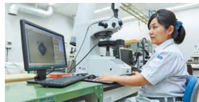
Hardness test using a Vickers hardness tester
