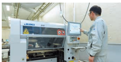
Durability test for a chip mounter
