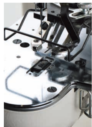
Mechanism for shortening leftover thread in the LK-1903BB
