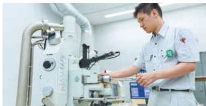
Elemental analysis using an EPMA
