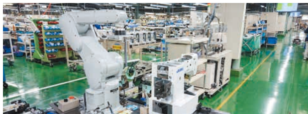
Robot attaching caution and warning labels to machines (at our Ohtawara plant)
