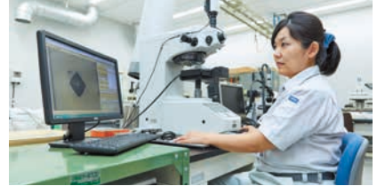
Hardness test using a Vickers hardness tester
