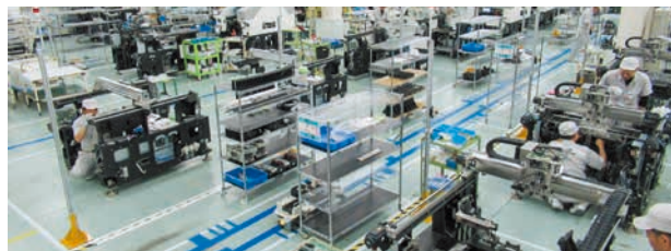
Takt-controlled production using the AGV (at JUKI Industrial Equipment Technology Corporation)
