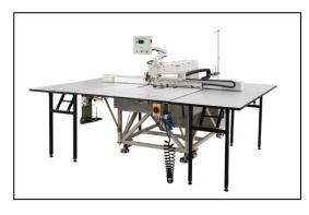
runstitching many parts such as shirt cuffs also in a single sewing sequence. Normally, the sewing machine that has a large sewing area requires frequent change of bobbin thread. For the PS-700, however, the bobbin changer (BK-7) feature is available to solve the inconvenience of frequent bobbin
