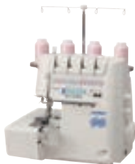
Overlock with air-supported threading MO-1000
