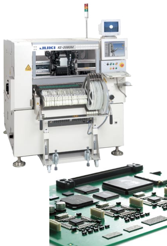
General-purpose chip placement machine that can be used for a range of parts
