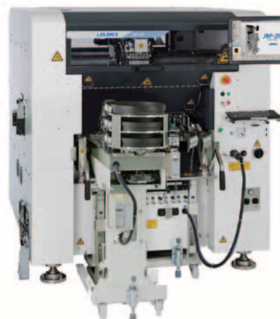
JM-20 realizes automation of the manual component insertion process
