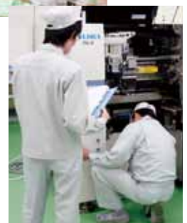
Maintenance and inspection of a pick and placer(SMT)
