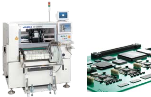
General-purpose pick and placer usable for a range of different parts
