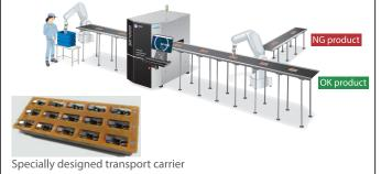
Labor saving: reduces the number of personnel in the inspection process from 4 to 1, improving the overall inspection quality. And establish traceability.
