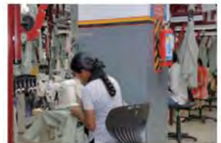
2-Needle Double Stitch Machine used for shirt shoulder MS-1190M
