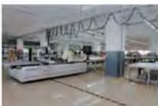
Cutting Machine moves on the rail paved on the floor
