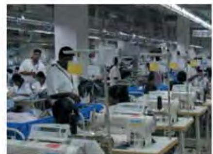
Mainly DDL-9000 series on production line
