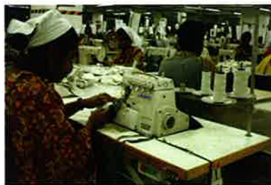
② High speed safety stitch machine, the MO-6716S.
