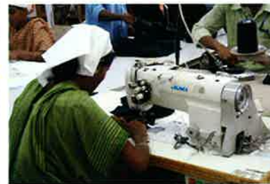
③ 2-needle needle-feed lockstitch machine, the LH-3128. Various gauges are provided for light-weight material, heavy-weight material or jeans/heavy-weight material. Operators praise this machine because of its adaptability to different materials.
