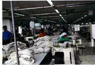
As far as you can see, all sewing machines are JUKI. The latest sewing machines are introduced for the lockstitch, mainly the DDL-8700 with an automatic thread trimmer.
