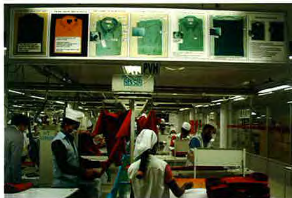
Hangers are used in the finishing line. Check points in the sewing finishing process for each product are shown on the ceiling above the operators' heads.
