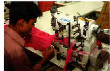
High speed cylinder-bed 3- needle top and bottom coverstitch machine, the MF-7823.
