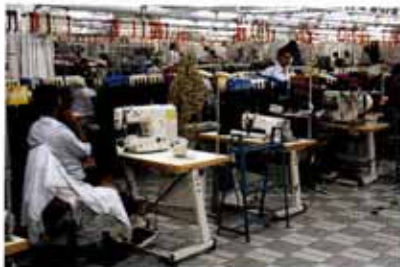
The factory is managed using a unique chain system using hangers. One line consists of approximately 50 operators with 2,000 hangers used in the line.
