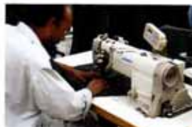
2-needle, Lockstitch machine with automatic thread trimmer and an organized split needle bar LH-3168-7 for double stitch
