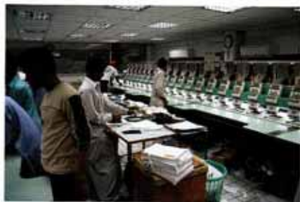
Multiple-head embroidering machines are also used effectively. They help increase the added value of the products.
