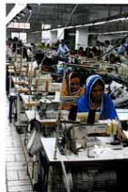
On the sewing line: Operators use 1-needle, lockstitch machines with automatic thread trimmers.
