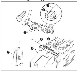
Set button 1 to button loader 2 and depress the back part of the pedal to insert the button into button chucks 3. (When the button loader is not used, insert the button by hand since the chuck is opened by depressing the back part of the pedal.)
