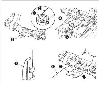
Set upper button ① to button loader ② and depress the back part of the pedal to insert the button into button chucks ③. (When the button loader is not used, insert the button by hand since the chuck is opened by depressing the back part of the pedal.)
