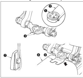
Set button 1 to button loader 2 and depress the back part of the pedal to insert the button into button chucks 3. (When the button loader is not used, insert the button by hand since the chuck is opened by depressing the back part of the pedal.)
