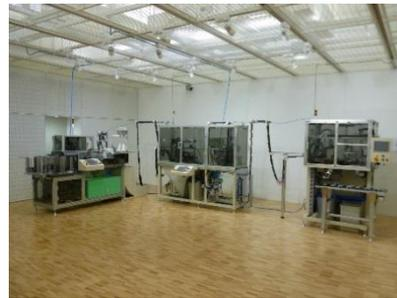
Left: A jeans fly and its location on a pair of jeans. Right: Machines to automatically align the zipper and the fly, and sew the zipper onto it as well as serge (sew) the edge of the fly.
