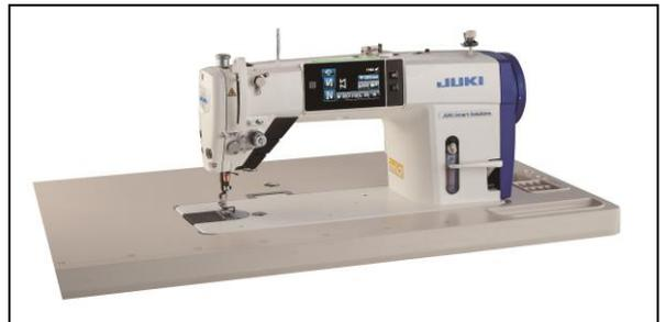
the operation panel. The sewing data that are best suited to materials of diversified products used in apparel sewing plants can be stored in memory on a material-by-material basis. In addition, the relevant data can be easily reproduced as desired when sewing under the same condition.
