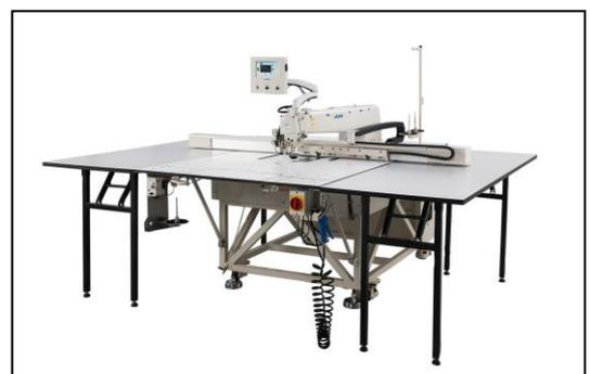
runstitching many parts such as shirt cuffs also in a single sewing sequence. Normally, the sewing machine that has a large sewing area requires frequent change of bobbin thread. For the PS-700, however, the bobbin changer (BK-7) feature is available to solve the inconvenience of frequent bobbin
