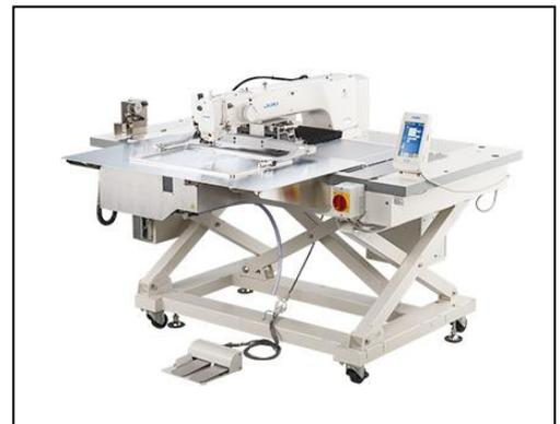
is able to concentrate on sewing without worrying about shortage of bobbin thread. In addition, only two bobbin cases are required for sewing. As a result, burdensome control of bobbin thread tension and bobbin-changing work are no longer required, thereby contributing to increased productivity.
