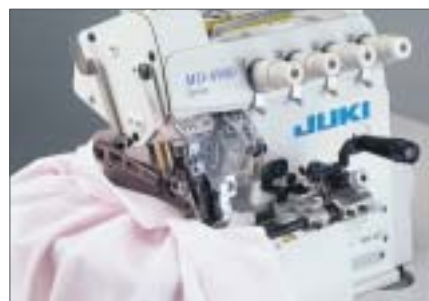
● For gathering MO-6914S-BE6-327/S162 (S162: Swing-type gathering device)
