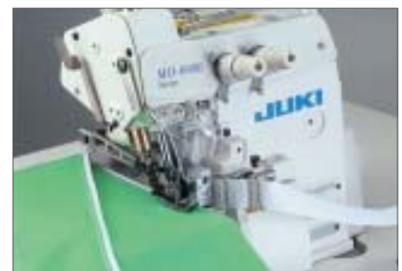
● For rolling-in tape MO-6945S-ED4-360/N077 (N077: Clean finish top and bottom)
