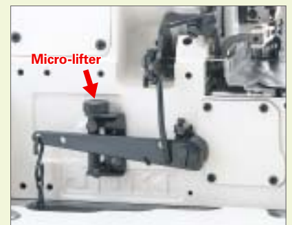
Bottom and top differential-feed micro adjustment mechanism
