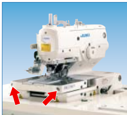
Material opening amount adjusting screw MEB-3200JS
