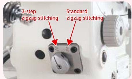
Standard/3-step zigzag stitching pattern changeover lever
