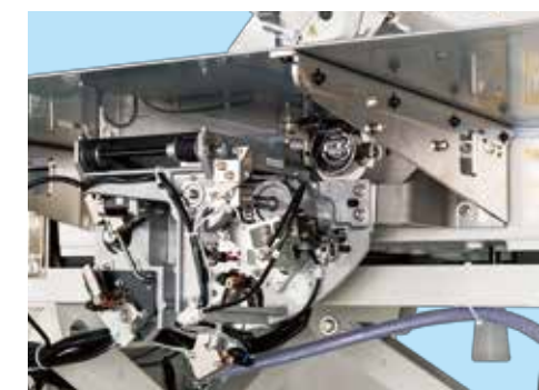
Automatic bobbin-thread winding and feeding unit
