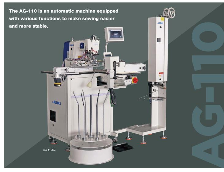
An automatic machine optimized for the ring processing of elastic waist braids for boxer shorts and briefs, equipped with various functions.
