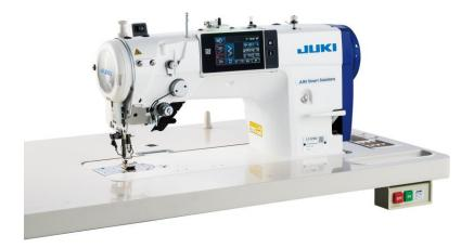
JUKI is going to launch "Semi-dry head, digital zigzag stitch sewing system, LZ-2290C Series" on May 21, 2019. The LZ-2290C Series has digitalized adjustment function for "sewing" not only to contribute to improved seam quality and reduced setup time but also to enable production management by combining JUKI exclusive software application with the sewing machine.
